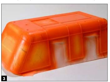
The interior color – international orange – is sprayed from the outside. The inside masking protects against overspray.
